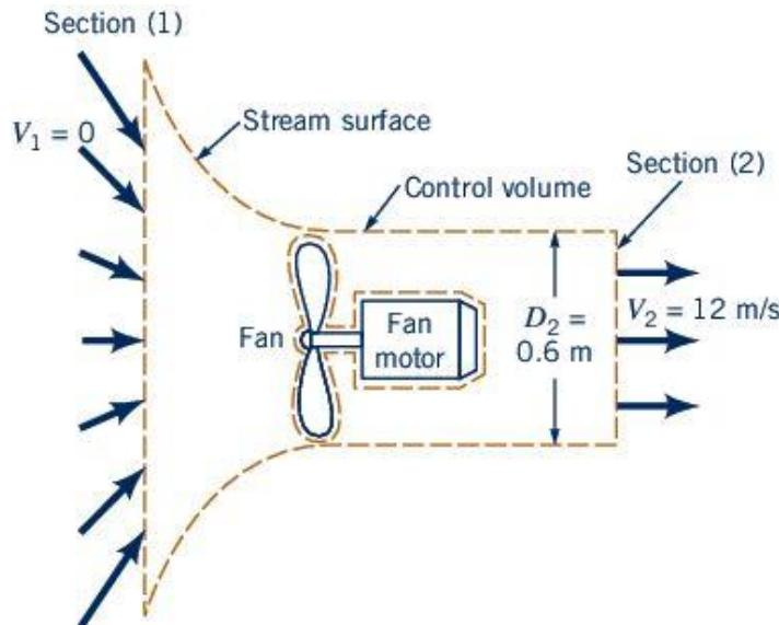
The fan delivers 0.4 kW to the blades. How much of the fan work produces useful effects, i.e. rise in energy? What is the fluid mechanical efficiency of the fan?
