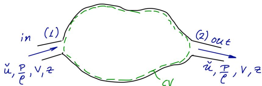
Special case: when there is only one stream entering and leaving the CV, and  $\check{u}, \frac{P}{\rho}, \frac{V^2}{2}, z$  are uniform over the inlet and outlet cross-sectional areas, then
