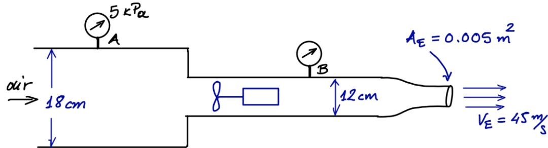
— Does the propeller act as a pump or as a turbine?
