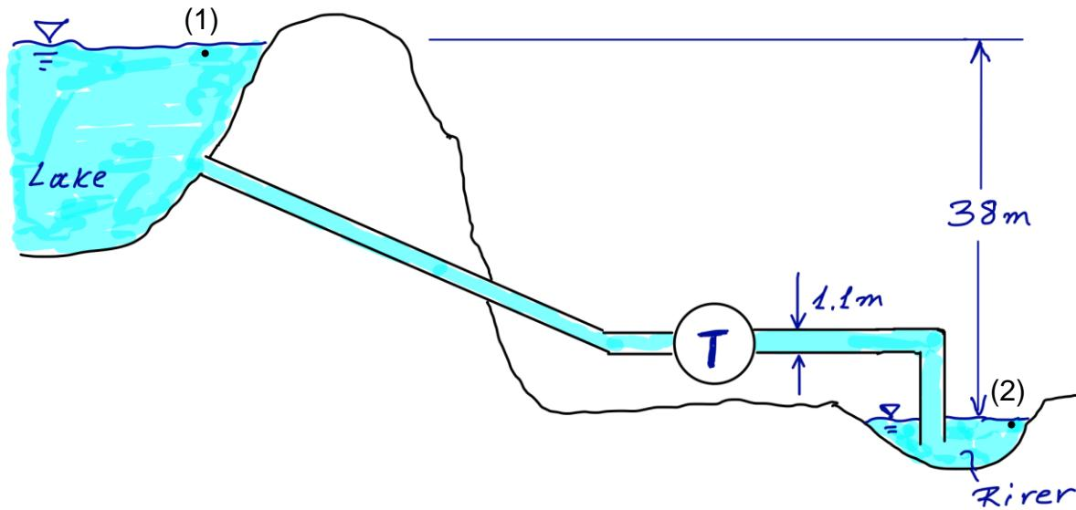
The turbine delivers to the generator 2.8 MW of power when the flowrate is  $Q = 15 \text{ m}^3/\text{s}$ .
